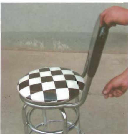
Step 7: Slide the backrest into the tubes, then bolt it.
