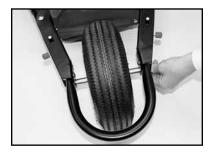
Step 5: Place the Wheel between the wheel axel and the Wheel Bracket. Insert the wheel axel through the wheel center and the second wheel space before inserting the axel through the hole on the Wheel Baracket. Hand tighten the nut and bolt to hold the wheel in place.
