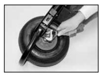
Step 6: Using an open end wrench or socket wrench tighten down all the nuts while appyling preasure to the head of the bolt making sure the tab on the bolt is in the notch on the frame so that the bolt sits flush frames surface. This will ensure a secure tightening and prevent the bolt from turning.
