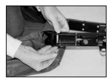
Step 2: Once the Handle is fed all the way through the sleeve remove the nut and bolt at the bottom of the sleeve to allow the Handle to be secured to the Wheel Bracket.
