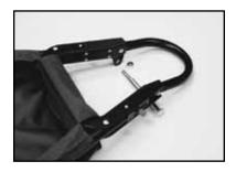
Step 4: Remove the nut holding the wheel axel in place and remove the axel about 1/2 from the Wheel Bracket. There should only be one (1) wheel spacer still on the axel.
