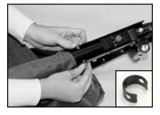
Step 3: Slide the Handle all the way down the sleeve and align hole on the Handle with the holes on the Wheel Bracket. Insert the bolt you removed in Step 2 throught the holes in the handle and Wheel Bracket paying close attention that the Protective Sleeve (insert) is still on the handle and habd tighten the nut to the bolt. Repeat for the other handle.
