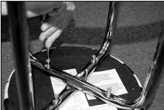
Step 3: Place the seat pad on a flat stable surface with the underside facing up. Turn the assembled legs and place it on the underside of the seat pad. Align the holes in the legs with the holes in the seat pad base. Using the supplied machine screws or self-tapping screws secure the seat pad to the legs.
