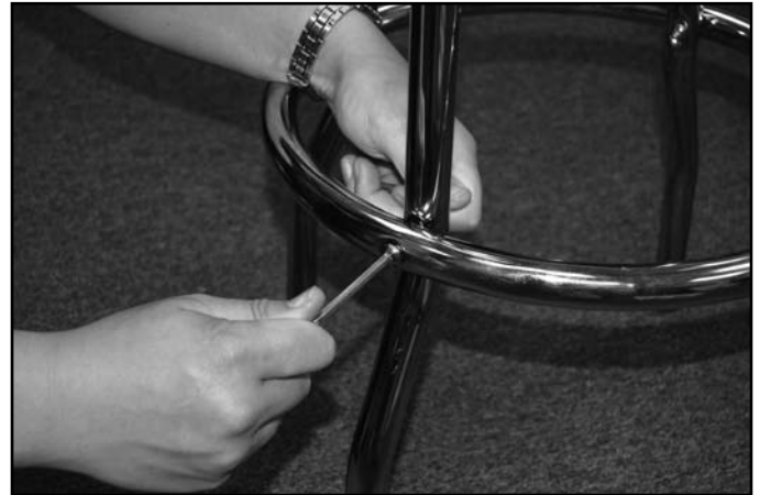
Step 2: Slide the ring over the legs and align the holes on the ring with the holes on the legs. Slide the sleeved, allen head screw into the hole and an allen head screw through the other side and tighten down using the supplied allen wrenches. Repeat for the other holes.
